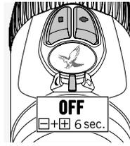
You can deactivate the SWAROLIGHT function by turning the OFF/DAY/NIGHT switch to the central position and pressing the +/- buttons at the same time for 6 seconds. The light will flash twice to confirm
