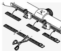
The cover provided can be used to protect the exposed areas of the rail. You can cut it to the required size and press it into the rail using your fingers.
