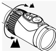
Turn the magnification adjustment ring through up to 180° to obtain the required magnification. The adjustment is continuous. The scale on the adjustment ring makes it easy to see the setting. The soft ribbed cover of the adjustment ring has a small protrusion to make orientation easier.
