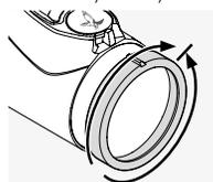
First, turn the diopter adjustment ring fully to the left (counter-clockwise) and then to the right until the reticle is in sharp focus. The adjustment range depends on the individual model.
