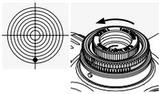
Turn the outer knurled ring on the top turret in the direction of H (counter-clockwise).
