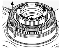
1. Lift the outer knurled ring and keep it in this raised position while turning it. It will not remain in the raised position of its own accord.
