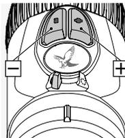
You can now adjust the brightness in the mode you have selected using the +/- buttons. To reach the ideal level of brightness quickly, you can press and hold one of the buttons (long pulse). To make precision adjustments, press either of the buttons once (single pulse).
