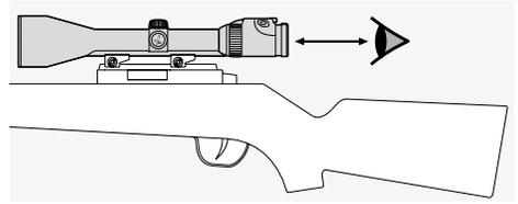
Set the eye relief correctly for a scope mounted on a firearm (see the technical data sheet for the measurements).
